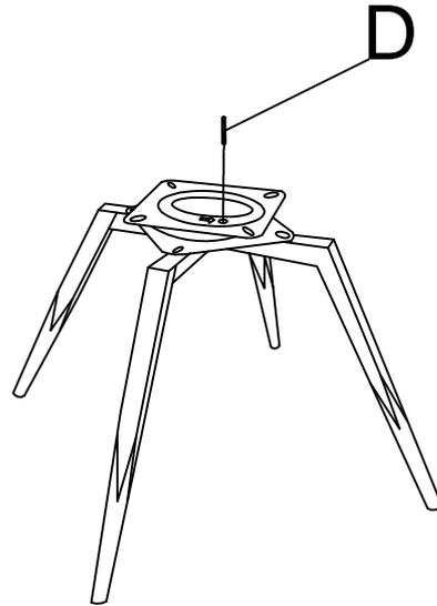
Turn around the rotate plate 45 degree
